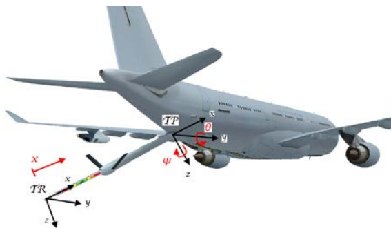
Figure 4 – Flying Boom Generalised Coordinates
